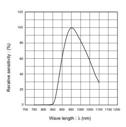
Fig.7 Optical bandwidth of the photo-diode encapsulation
