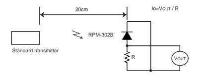
Fig.2 Measurement of standard transmitter proofreading
