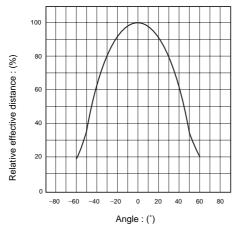
Fig.8 Direction characteristic (Horizontal direction)
