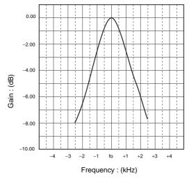
Fig.6 RPM7157 Series BPF Characteristics
